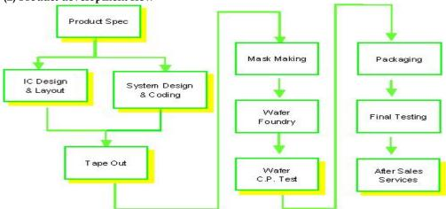
\*Blocks w/ shadows are in-house activities, and w/o shadows are subcontracted out. In the product development flow, Sunplus focus on IC design, system design, wafer testing and sales services but out-sources most aspects of the manufacturing including mask making, wafer fabrication, wafer sawing, packaging and final testing.
